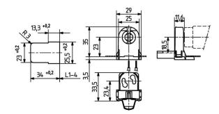
L1-4: Recommended dimension - The distance between the cutouts and the tolerance should be governed by the dimensions of the respective lamps and luminaires.
